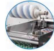
Web guide sensor with fine control knob
